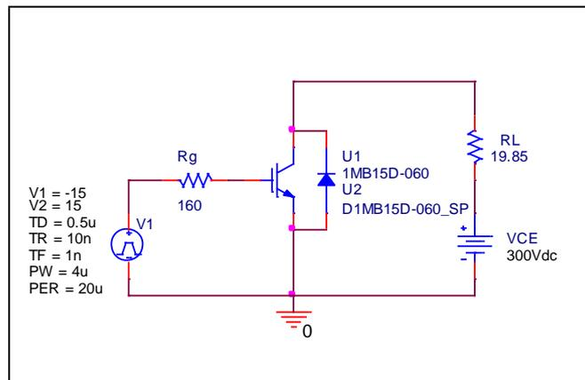
Test condition:  $I_C=15$  (A),  $V_{CC}=300$  (V)
