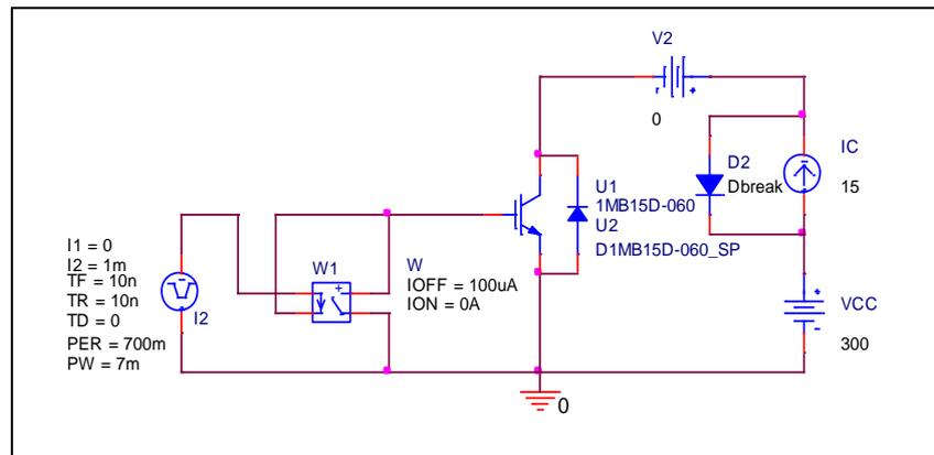
Test condition:  $V_{CC}=300$  (V),  $I_C=15$  (A),  $V_{GE}=15$  (V)
