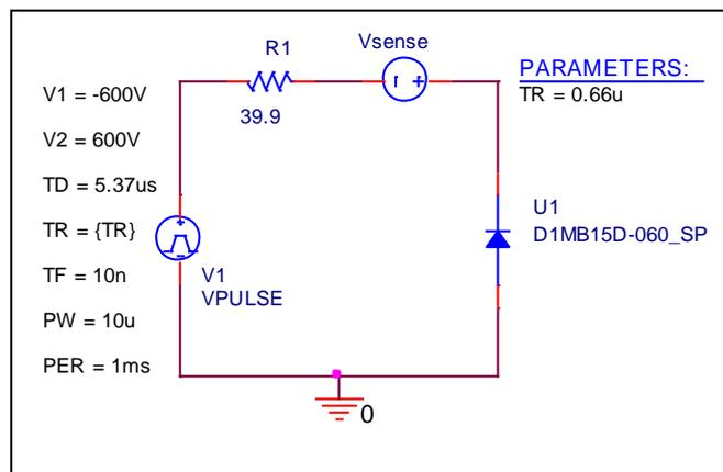
Test condition:  $V_{CC}=600$  (V),  $I_C=15$  (A),  $-di/dt= 45$  (A/us)
